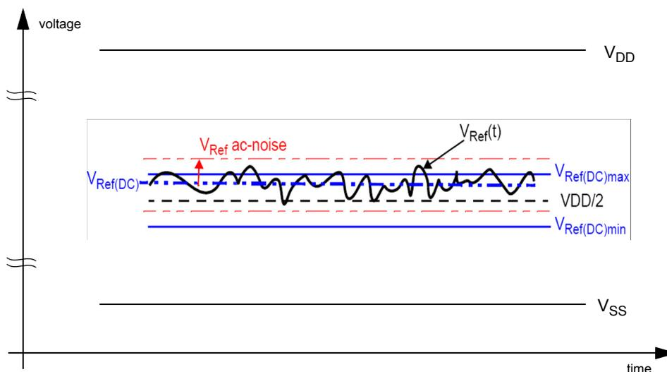
Figure 1. Illustration of V<sub>REF</sub>(DC) tolerance and V<sub>REF</sub> AC-noise limits
