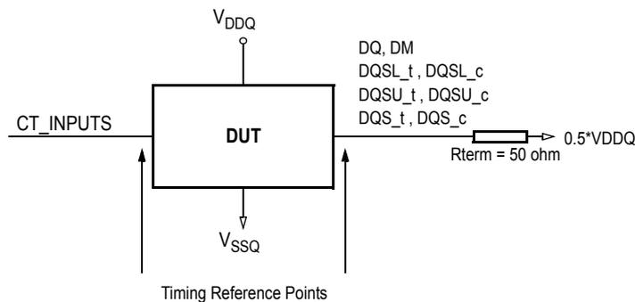
Figure 9. Connectivity Test Mode Timing Reference Load
