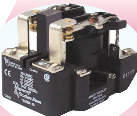
199B DPDT WITH MAGNETIC BLOWOUT FOR DC ARC QUENCHING 10 AMPS, 110 VDC
