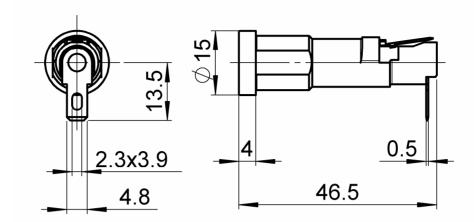
Flange form cylindrically, quick-connect terminals 4,8 x 0,5mm white solder hole 3.9 x 2.3mm, 90° end terminal
