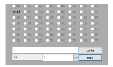
Selecting address 48 and clicking on **read** reads a single byte from the temperature sensor. The  $I^2CDriver$  display shows the traffic immediately.
