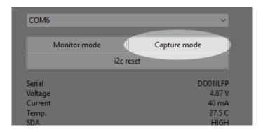
Clicking "Capture mode" starts the capture and prompts for a destination CSV file. The character in the top-left of the display changes from D to C. Capture
