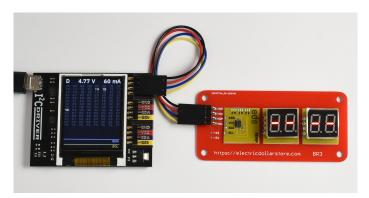
Starting the GUI and connecting to the  $I^2CD$ river on COM16 shows the temperature sensor at address 48 and the two display modules at addresses 14 and 15.
