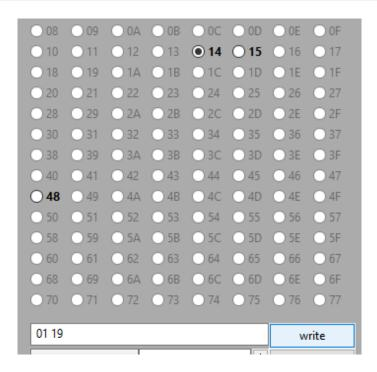
Selecting the left-hand display (address 14) and entering the hex values 01 19 then clicking on **write** sets the first LED to the digits 19.
