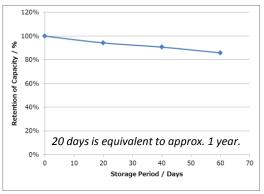
Measurement conditions: Temp: 23 deg C Storage conditions: 60 deg C Dry Load:  $30k\Omega$
