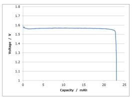
Measurement conditions: Temp: 23 deg C Load:  $30k\Omega$
