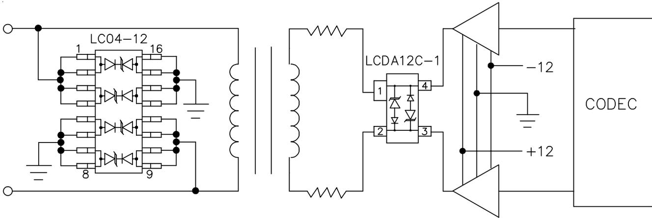
Figure 3 - ADSL Protection (Remote Terminal)
