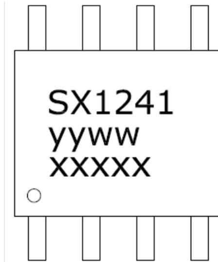
Figure 2. Marking Diagram
