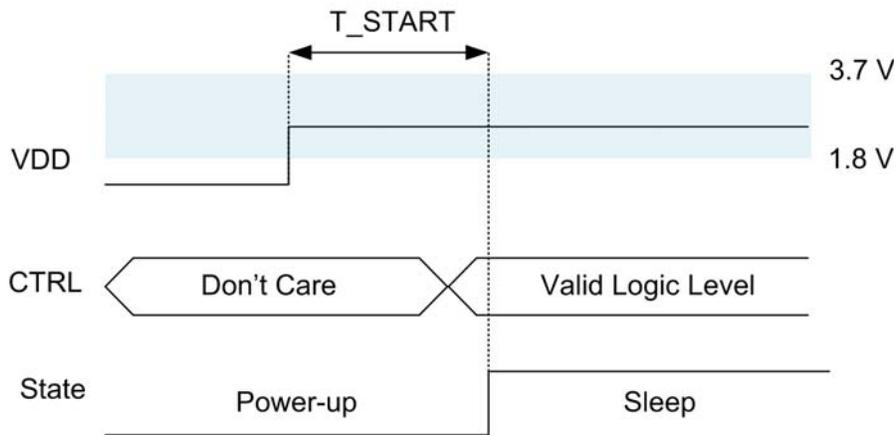
Figure 7. Power-up Timing
