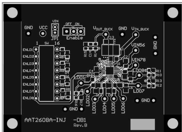
Figure 2: AAT2608A Evaluation Board Top Side PCB Layout.
