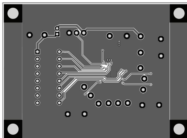
Figure 3: AAT2608A Evaluation Board Bottom Side PCB Layout.
