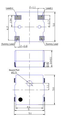
All dimensions are in mm Tolerance: **±**0.2 mm
