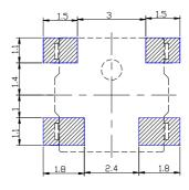
All dimensions are in mm, Tolerance: £0.2 mm
