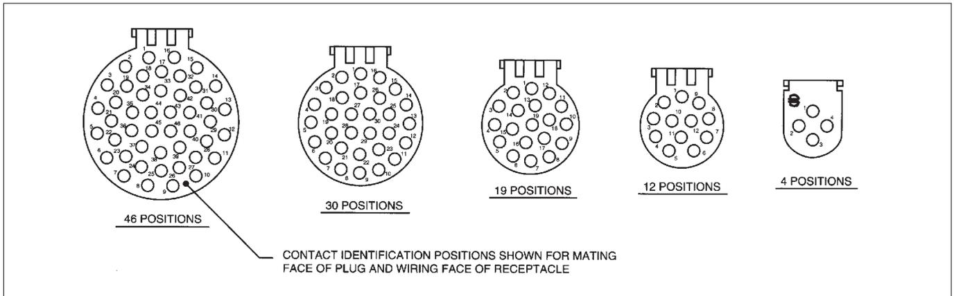
Contact identification positions shown are for mating face of plug and wiring face of receptacle.
