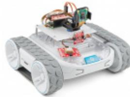
SparkFun Advanced Autonomous Kit for Sphero RVR
