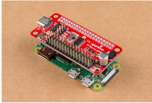
*Pi Servo pHAT properly connected to a Raspberry Pi. Click image to enlarge.*
