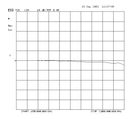
Insertion loss tested to 7 GHz for the CRFReed Relay but with the internal Reed Switch replaced with a bare copper wire. Horizontal full scale: 7.0 GHz. Vertical scale: 10 dB/div referenced from the 0 mark.
