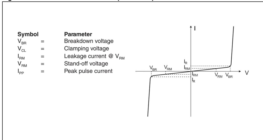
**Table 2. Electrical characteristics (values,  $T_{amb} = 25\text{ °C}$ )**
