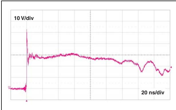
Figure 9. ESD response to IEC 61000-4-2 (-8 kV contact discharge) on each channel
