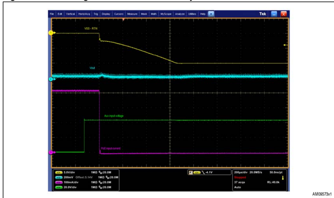
Figure 18. Switching between PoE and auxiliary source
