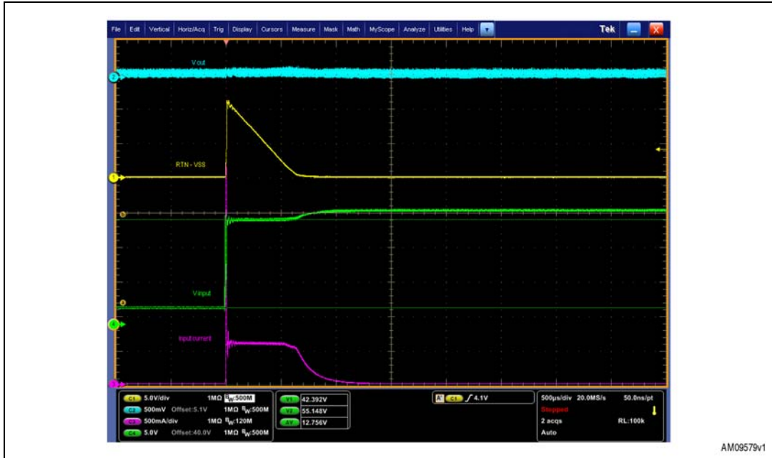
Figure 24. Effect of a 12 V line transient on the converter at 0 A load
