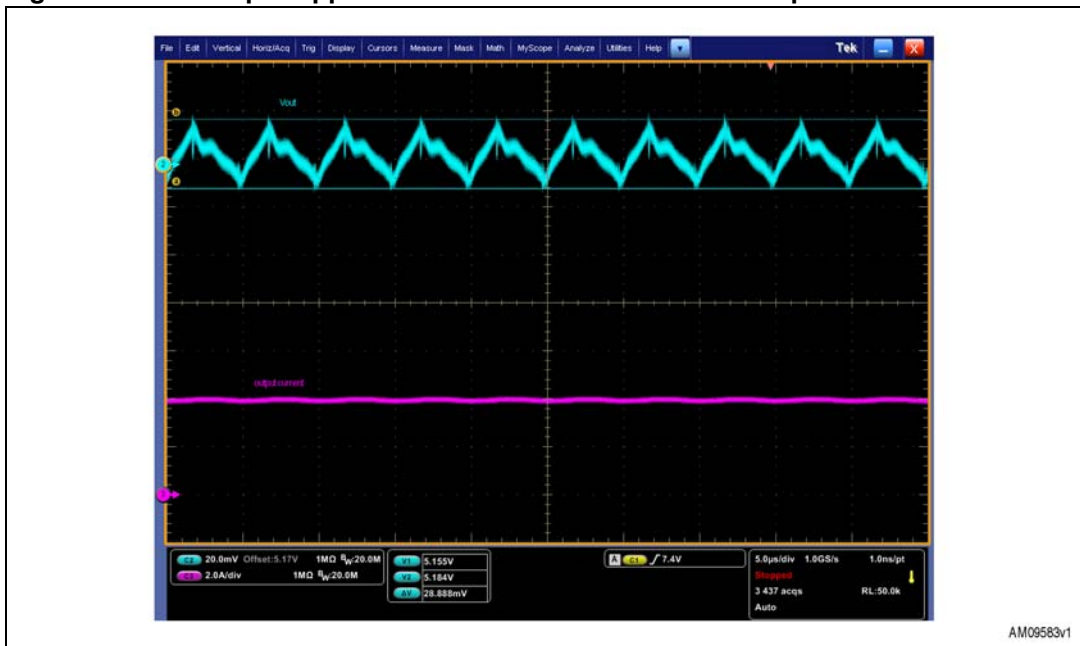
Figure 28. 5 V output ripple measurement at 4 A with infinite persistence
