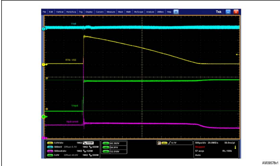
Figure 23. Effect of a 12 V line transient on the converter at 4 A load
