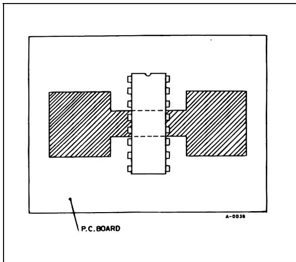
Figure 4 : Example of an External Heatsink
