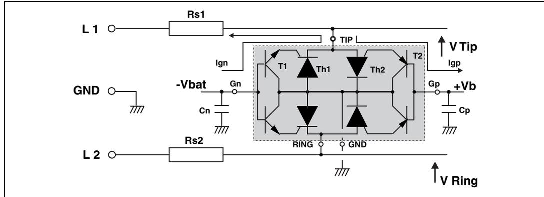
Figure 7 shows the classical protection circuit using the LCP12 crowbar concept. This topology has been developed to protect the new two-battery voltage SLICs. It allows both positive and negative firing thresholds to be programmed. The LCP12 has two gates (Gn and Gp). Gn is biased to negative battery voltage  $-V_{bat}$ , while Gp is biased to the positive battery voltage  $+V_b$ .
