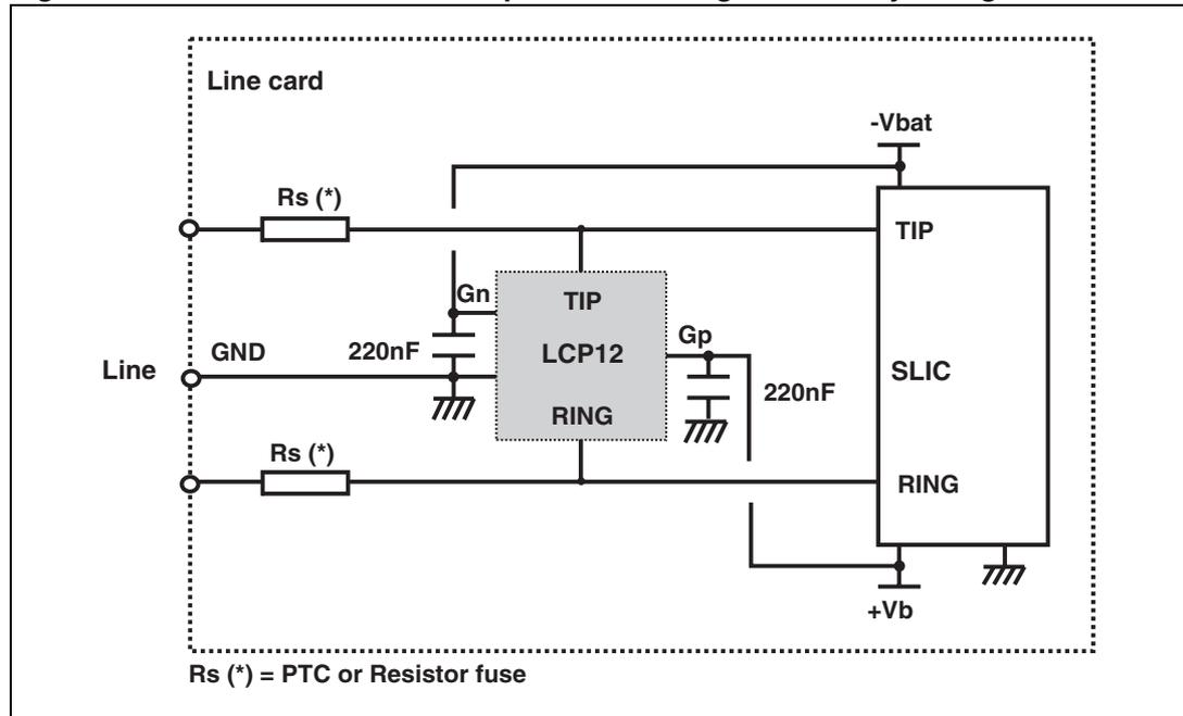
[Figure 8](#) shows the classical protection topology for SLIC using both positive and negative battery voltages. With such a topology the SLIC is protected against surge over +V<sub>b</sub> and lower than -V<sub>bat</sub>. In this case, +V<sub>b</sub> can be programmed up to +120 V while -V<sub>bat</sub> can be programmed down to -120 V.
