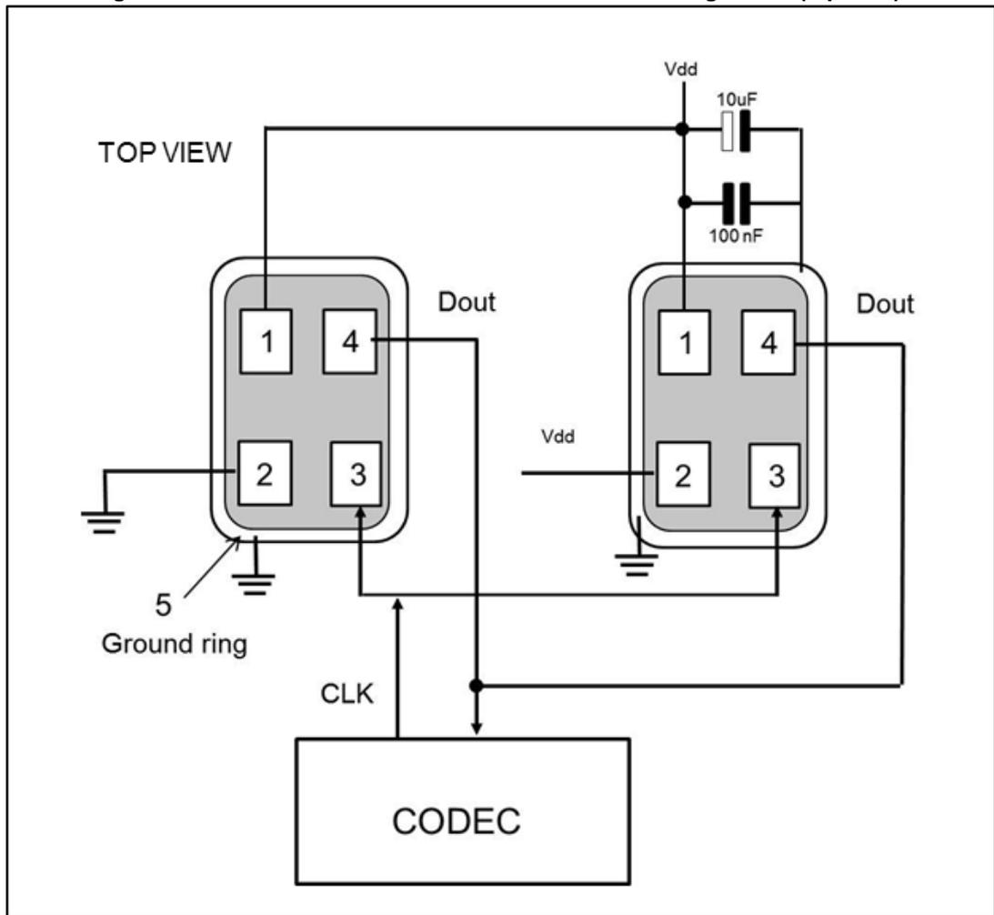
Power supply decoupling capacitors (100 nF ceramic, 10 µF ceramic) should be placed as near as possible to pin 1 of the device (common design practice).
