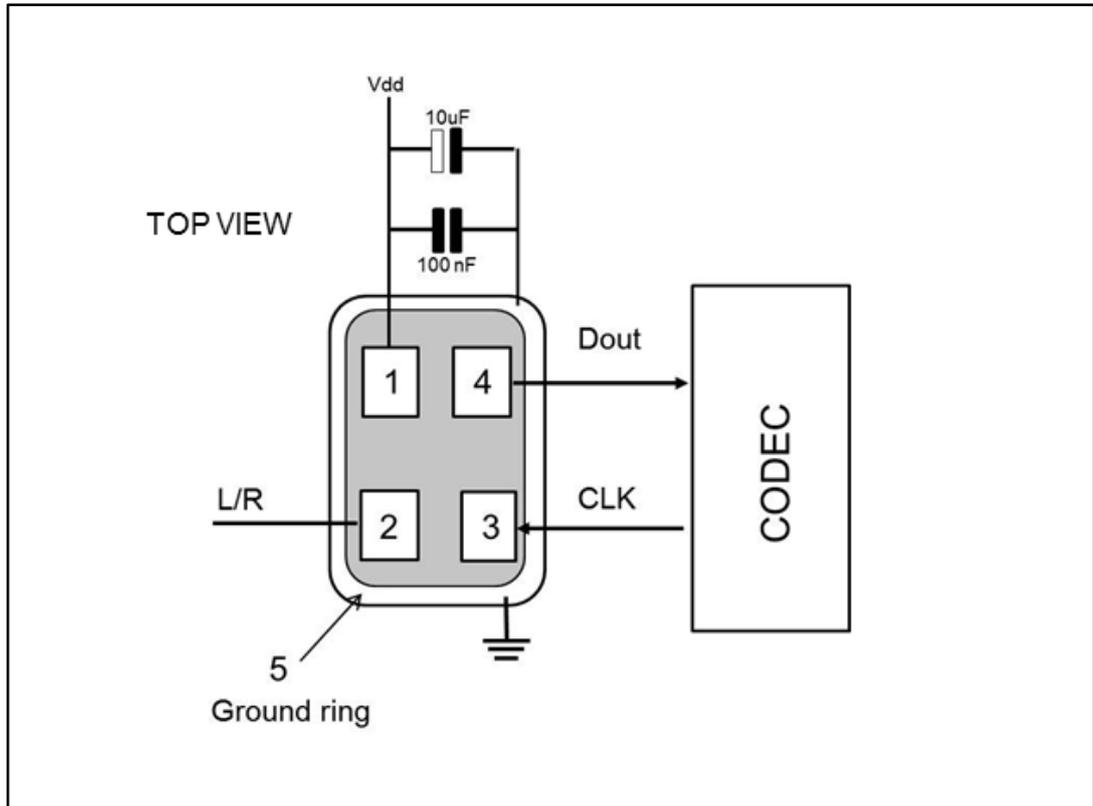
Figure 5: MP34DT04 electrical connections for stereo configuration (top view)
