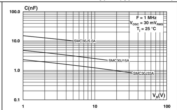
**Figure 7. Junction capacitance versus reverse applied voltage for bidirectional types (typical values)**
