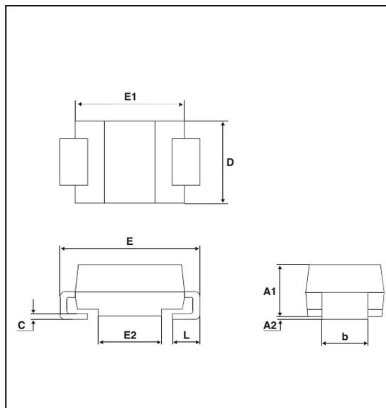
**Figure 13. Footprint dimensions mm (inches)**
