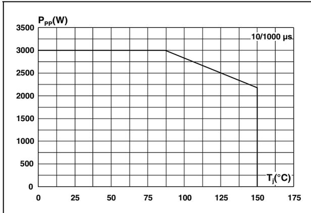
**Figure 4. Peak pulse power versus exponential pulse duration (T<sub>j</sub> initial = 25 °C)**
