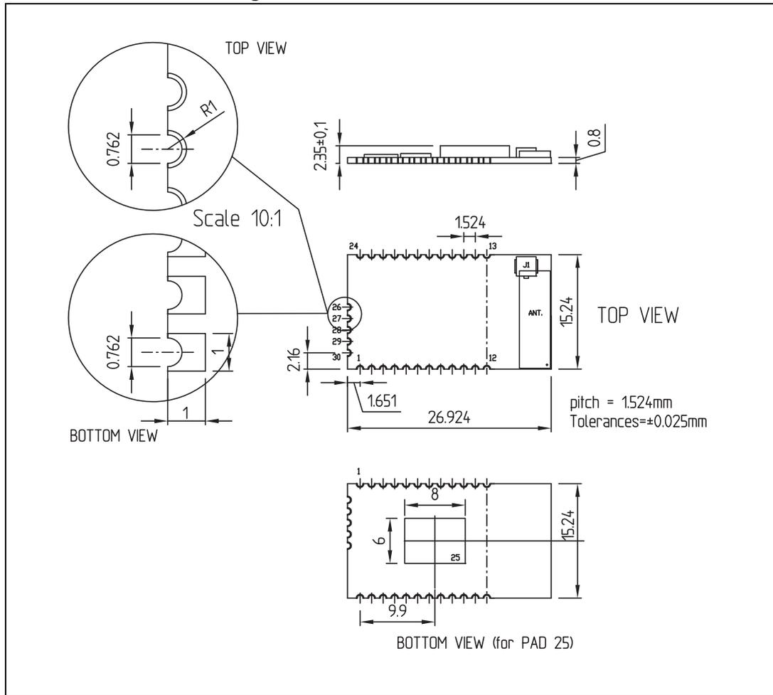
**Note:** An antenna area of 217 x 520 mils must be free of any ground metalization or traces under the unit. The area extending away from the antenna should be free from metal on the PCB and housing to meet expected performance levels. Pin 25 is the required paddle ground and is not shown in this diagram.
