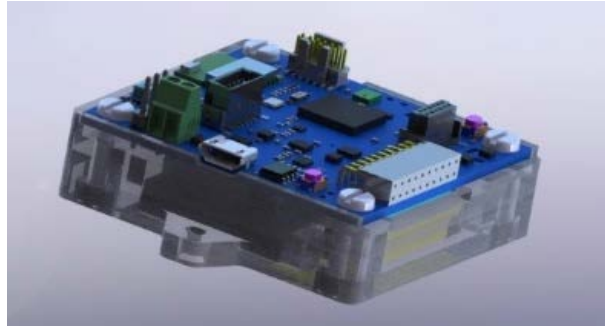
Figure 26. Core system board fastened with bolts
