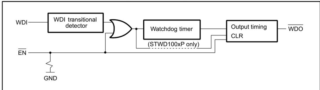
1. If the positive pulse on the enable pin,  $\overline{EN}$ , is longer than 1  $\mu\text{s}$ , it resets the watch.
