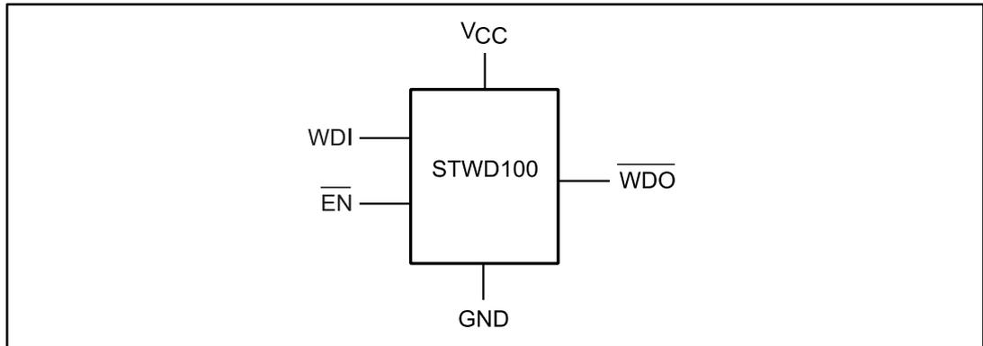
1. The  $\overline{WDO}$  output is available *in open drain or push-pull configuration*.
