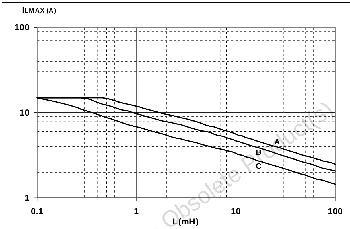
Figure 27. Maximum turn off current versus load inductance
