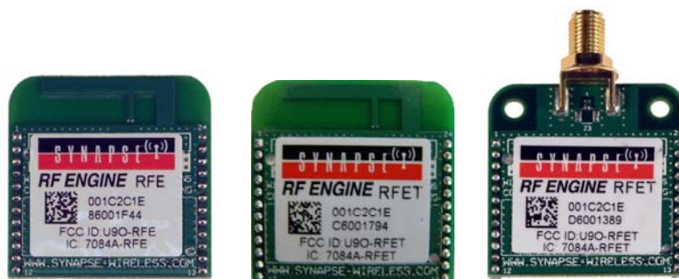
Figure 2 - The Synapse RFE, RFET, and RFET with external antenna engines
