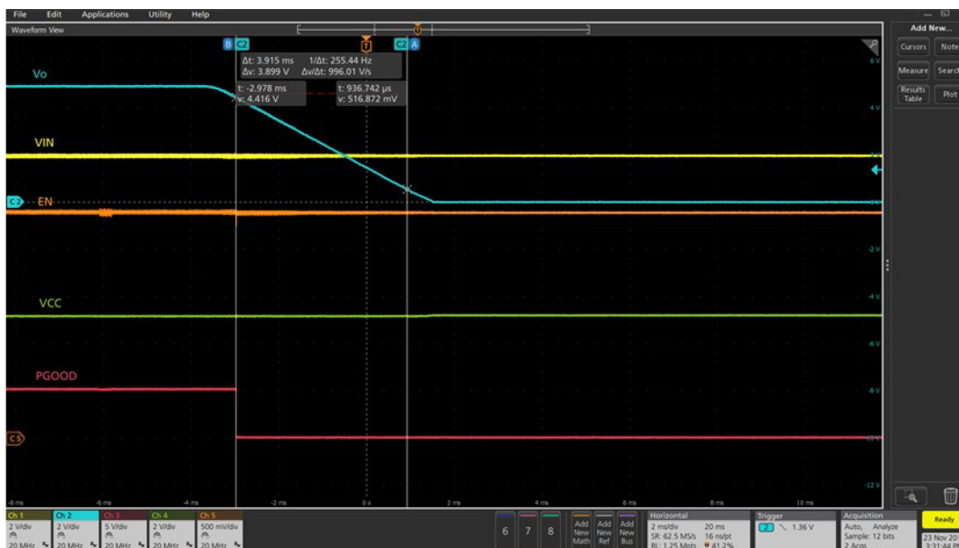
Figure 19 Soft turn off at 3A load (Ch1:PV IN , Ch2: V OUT , Ch3: PGood, Ch4:V CC , Ch5: Enable)
