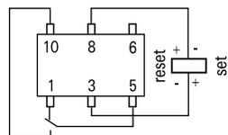
Latching type, 2 coils reset condition
