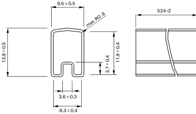
Tape and reel for SMT version - 480 relays per reel, 2400 per box
