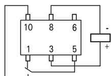
Latching type, 1 coil reset condition
