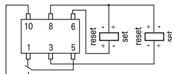
Contacts are shown in reset condition. Both coils can be used either as set or reset coil.
