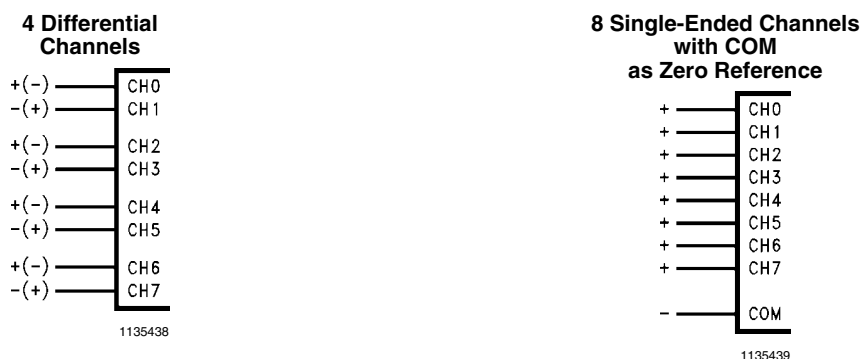
FIGURE 9. Input Multiplexer Options
