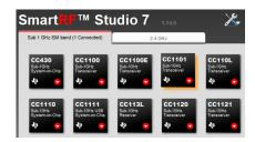
Launch SmartRF Studio and double click on the highlighted CC1101 device icon to get complete control of the device from the PC.
