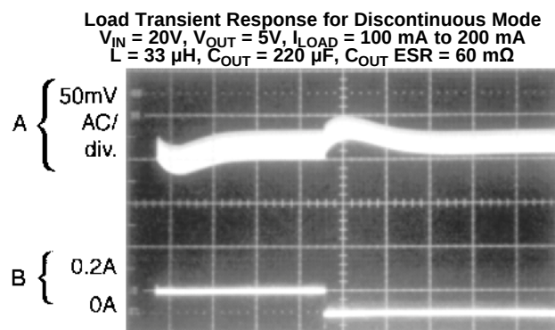
Figure 23. Horizontal Time Base: 2 \mu\text{s} /div.
