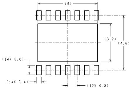
DIMENSIONS ARE IN MILLIMETERS
