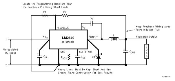
FIGURE 2. Basic circuit for adjustable output voltage applications
