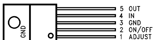
Figure 8. TO-220 5-Lead Power Package Front View
