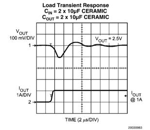
**Load Transient Response**  $C_{IN} = 2 \times 10 \mu F$  CERAMIC  $C_{OUT} = 2 \times 10 \mu F$  CERAMIC V<sub>OUT</sub> @ 2.5V I<sub>OUT</sub> @ 1A 2
