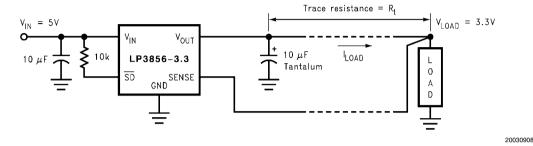
FIGURE 4. Improving remote load regulation using LP3856
