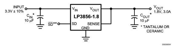
\*\* $\overline{SD}$  pin must be pulled high through a  $10k\Omega$  pull-up resistor. See Application Hints for more information.
