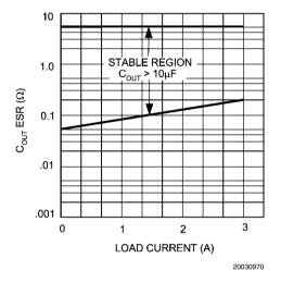
FIGURE 1. ESR Curve for C<sub>OUT</sub> (with 10µF Tantalum Input Capacitor)
