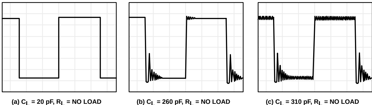
Figure 112. Effect of Capacitive Loads in Low-Bias Mode
