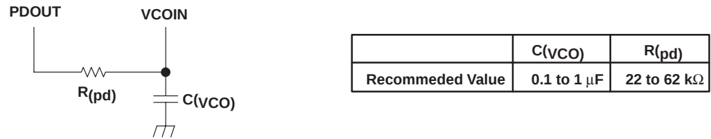
Figure 8. Resistor and Capacitor Connection
