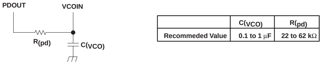
Figure 8. Resistor and Capacitor Connection
