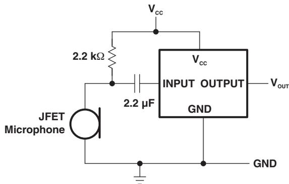
Figure 6. External Preamplifier
