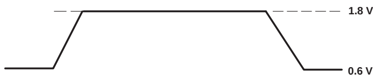
Figure 9. 'LC31 Input Levels
