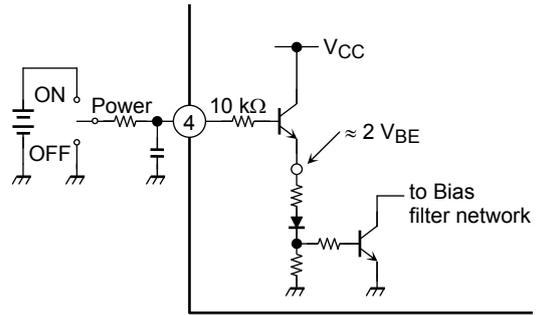
**Figure 1 Setting Pin 4 High Turns on Power**
