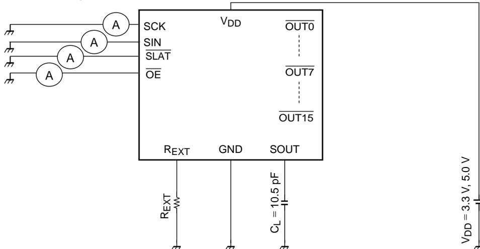
Test Circuit4: Power supply current
