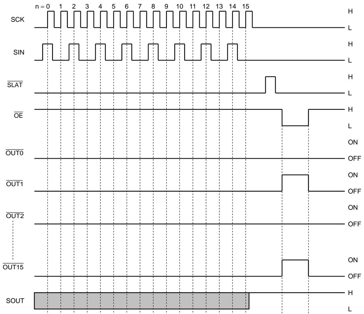
Note 1: The latch circuit is a leveled-latch circuit. Please note that it is not a triggered-latch circuit.
