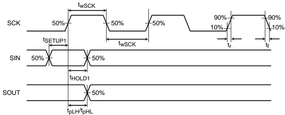
**2. SCK, SIN,  $\overline{SLAT}$ ,  $\overline{OE}$ ,  $\overline{OUT0}$**
