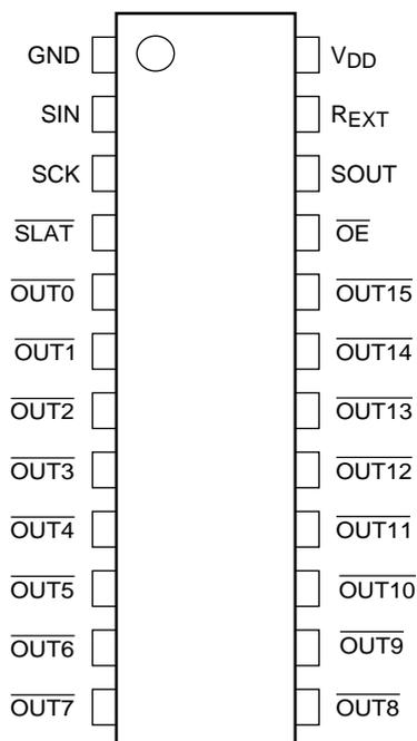
Note1: Short circuiting an output pin to a power supply pin (V<sub>DD</sub> or V<sub>LED</sub>\*), or short-circuiting the R<sub>EXT</sub> pin to the GND pin will likely exceed the rating, which in turn may result in smoldering and/or permanent damage. Please keep this in mind when determining the wiring layout for the power supply and GND pins.
