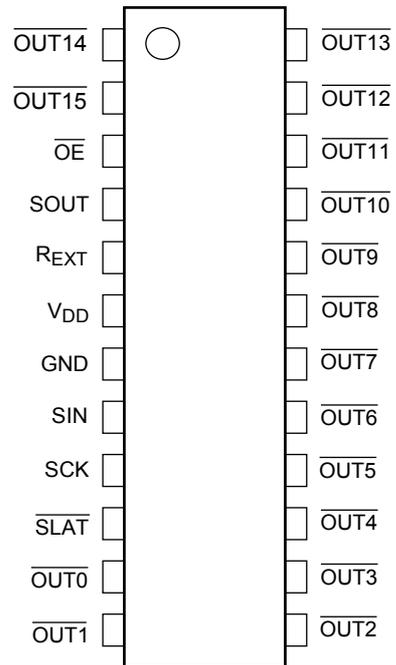
Note1: Short circuiting an output pin to a power supply pin (V<sub>DD</sub> or V<sub>LED</sub>\*), or short-circuiting the R<sub>EXT</sub> pin to the GND pin will likely exceed the rating, which in turn may result in smoldering and/or permanent damage. Please keep this in mind when determining the wiring layout for the power supply and GND pins.
