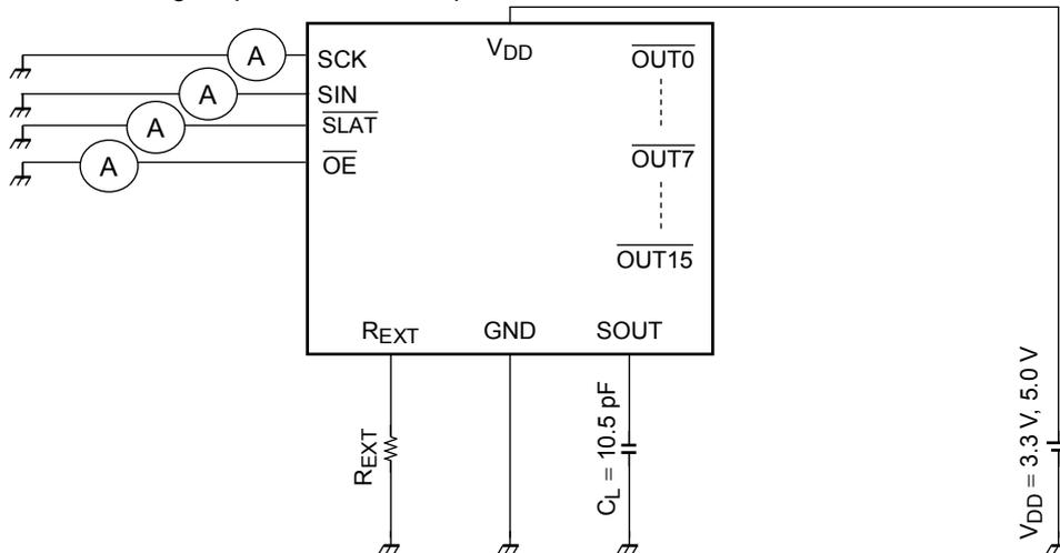
Test Circuit4: Power supply current
