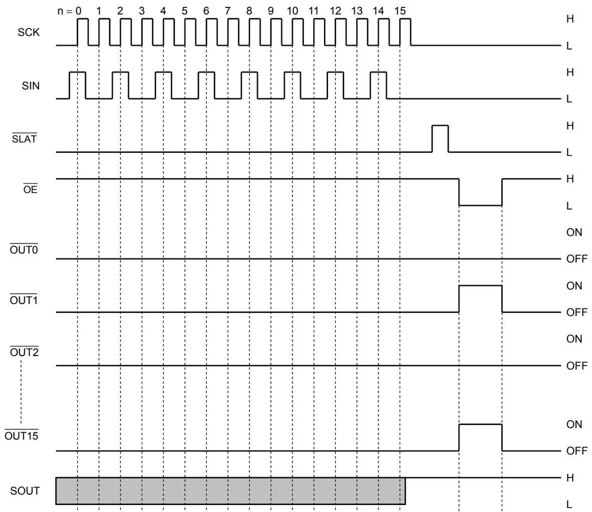
Note 1: The latch circuit is a leveled-latch circuit. Please exercise precaution as it is not triggered-latch circuit.
