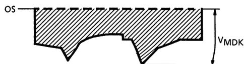
Note 6: Definition of DR :  $DR = \frac{V_{SAT}}{V_{MDK}}$
