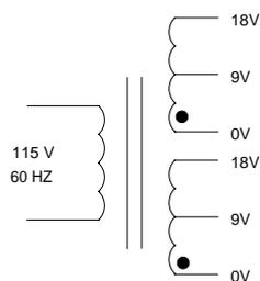
\* Secondary windings are designed to be connected in series or parallel. Windings are not intended to be used independently.
