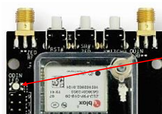
Figure 8: ODIN-W2 Activity LED position on C099-F9P board
