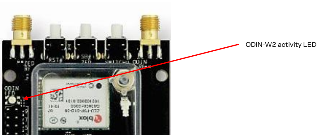
Figure 8: ODIN-W2 activity LED position on C099-F9P board
