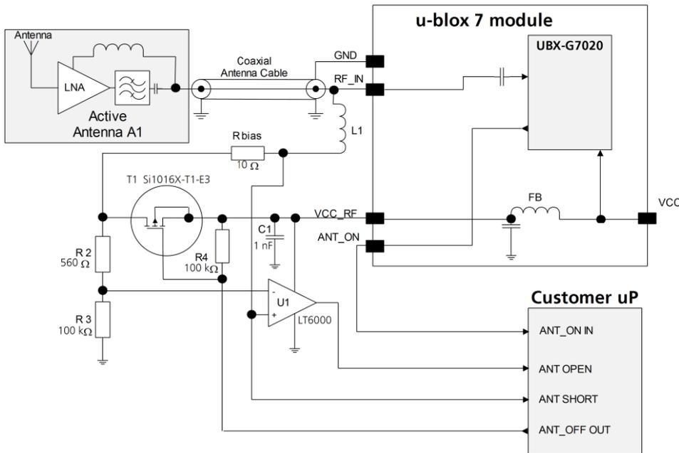
Figure 25: External active antenna supervisor using ANT\_ON
