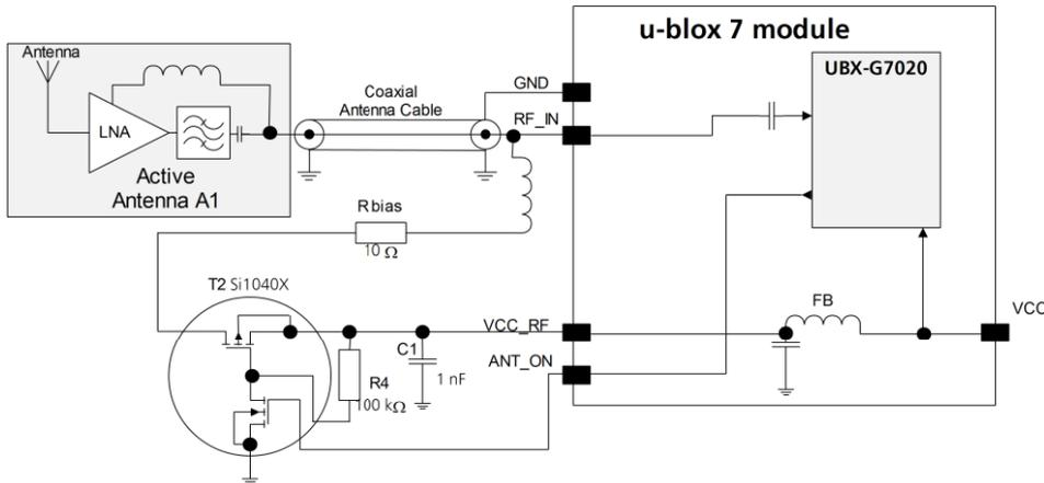
Figure 26: External active antenna control (MAX-7Q / MAX-7C)
