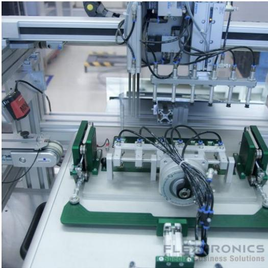
Figure 39: Automatic Test Equipment for Module Tests
