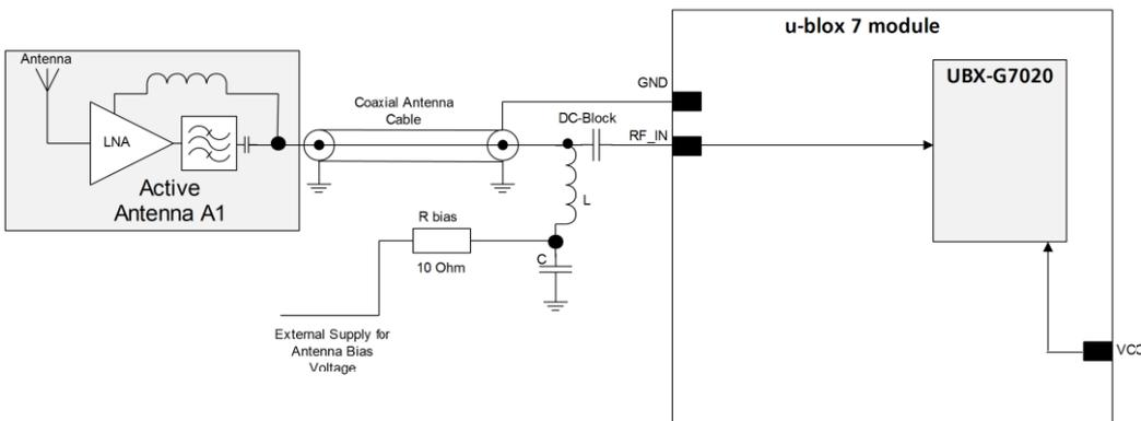
Figure 20: Active antenna design, direct external supply
