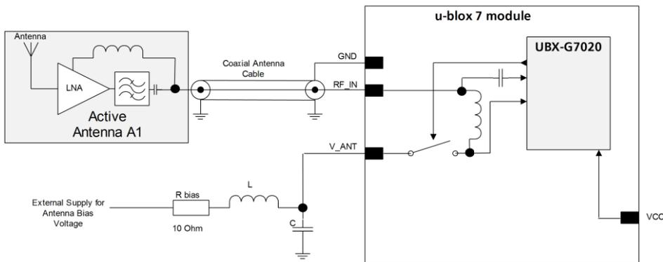
Figure 23: Module design with active antenna, external supply
