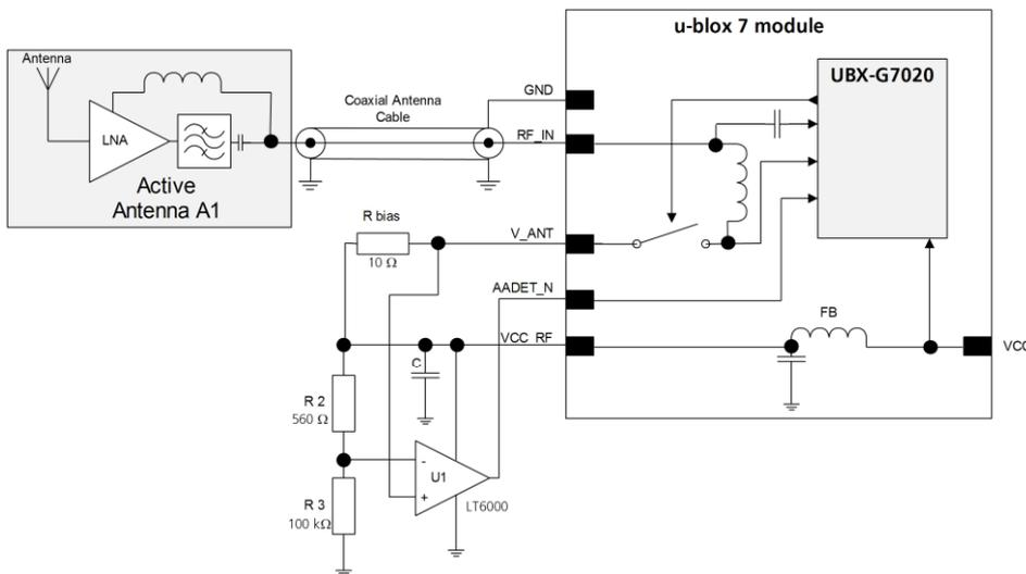
Figure 24: Schematic of open circuit detection
