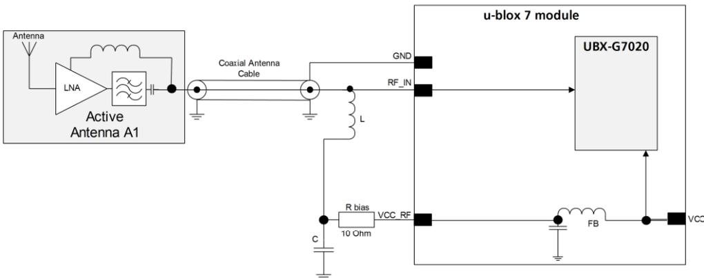
Figure 19: Active antenna design, external supply from VCC\_RF
