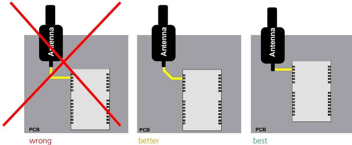
Figure 14: Recommended micro strip routing to RF pin
