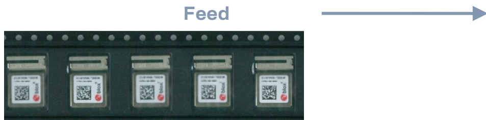
Figure 8: Orientation of NINA-B222 module on tape
