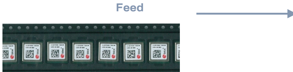
Figure 7: Orientation of NINA-B221 module on tape
