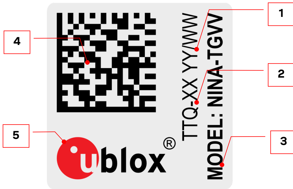
Figure 11: Location of product type number on the NINA-W13 series module label
