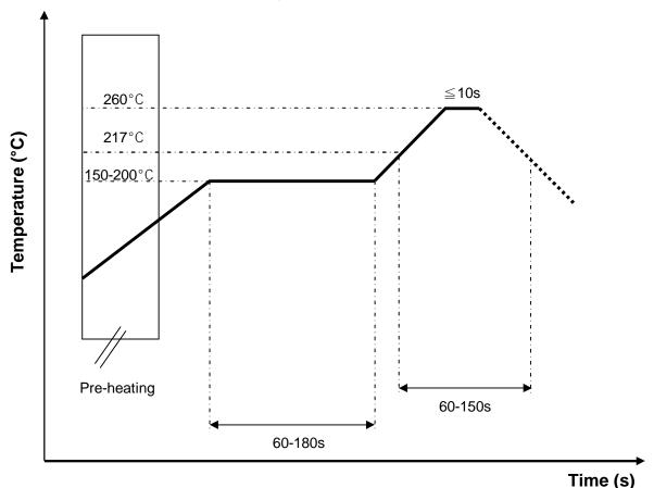
\*Recommended solder paste alloy: SAC305 (Sn96.5 /Ag3 /Cu0.5) Lead Free solder paste
