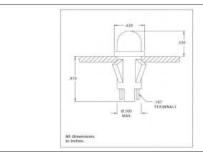
Part Number: 1051QA3 Serial Number: 1051 Light Source: Neon Color: Amber Voltage (V): 250VAC Mounting Hole (inch): 0,50 Mounting Hole (metric): 7,9 Termination: .187" QC Bezel color: Stainless Steel Housing color: White UL file: E20325
