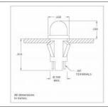
Part Number: 1090QA5-28V Part Number: 1090QA5-28V Serial Number: 1090 Light Source: Incandescent Color: Green Voltage (V): 28V Mounting Hole (inch): 0,50 Mounting Hole (metric): 12,7
