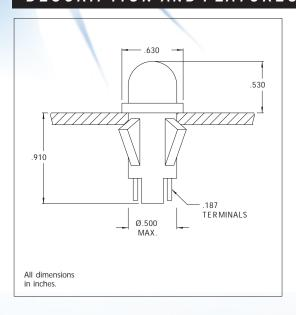
Mounting: Will snap-fit into Ø.500/.505 hole in panels .020/.100 thick. Push-on speednut SN0461 also available.
